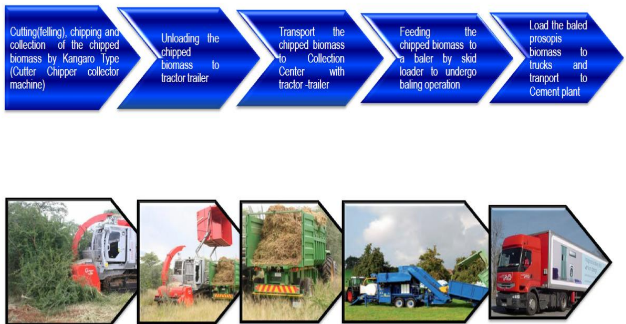
Figure 7:Process Flow Diagram for Fully Mechanized System of Harvesting, Baling and Transportation
