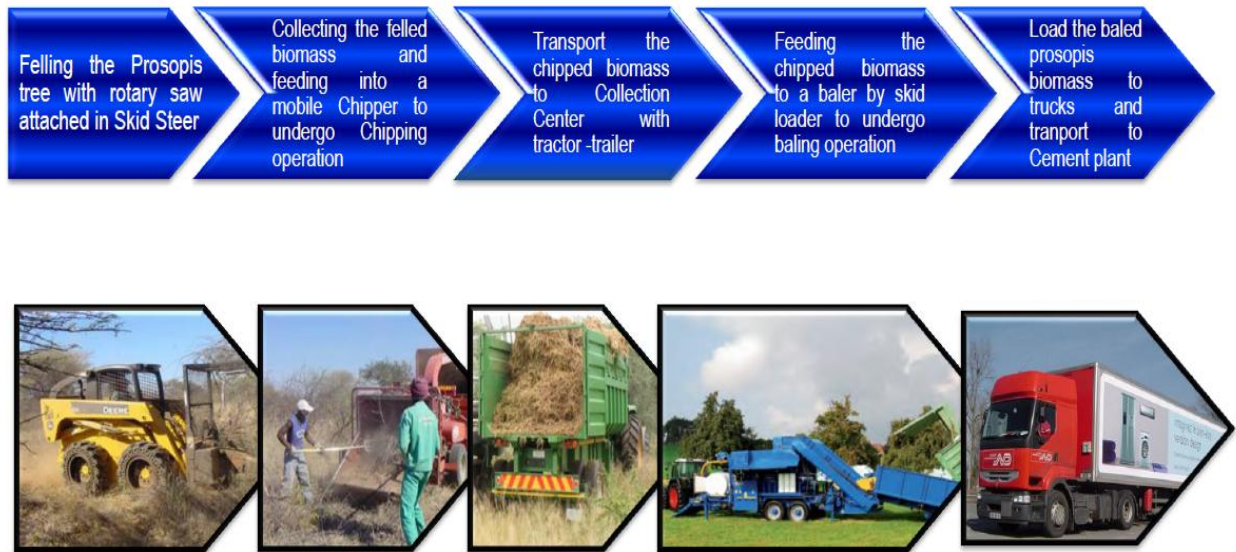
Figure 6: Process Flow Diagram for Semi-Mechanized way of Harvesting, Baling and Transportation
