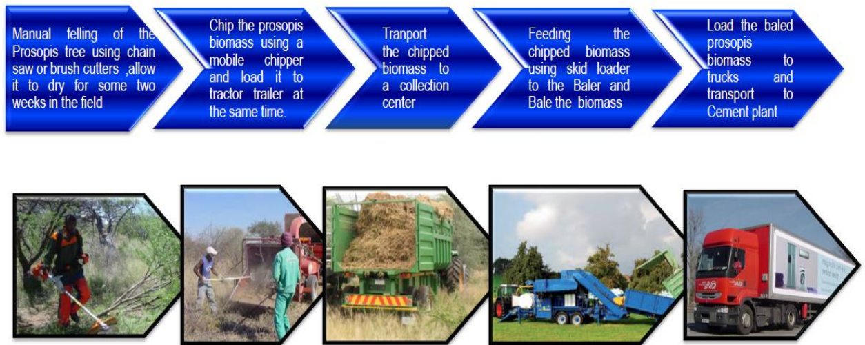
Figure 5: Process Flow Diagram for Semi-Manual Method of harvesting, baling and transportation
